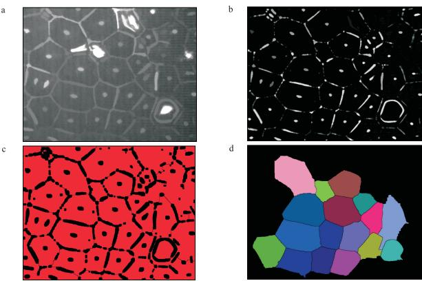
Fig. 3. a – result of erosion, reconstruction, dilation and opening operators; b – difference between source image and the image form the Fig. 3a; c-binarisation and transformation into convex areas using the distance function; d-the watershed operator finds and labels the cells.
