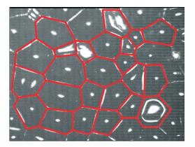
Fig. 4. Source image and manual sketching of the cell structure. The red lines were drawn on a separate layer.
